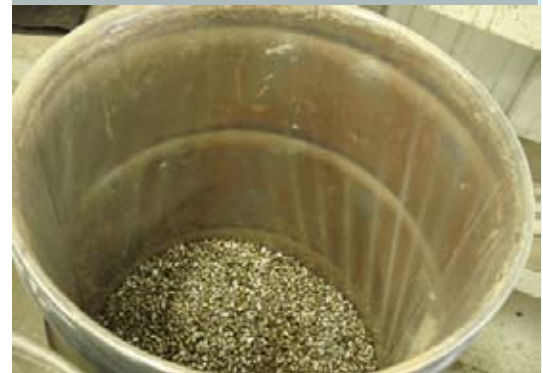
Mercury pellets removed from convenience light assemblies at EQ.
